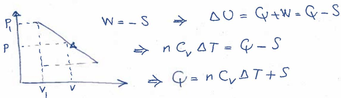
$$\Rightarrow Q = \frac{7}{2} n R (T - T_1) + \frac{1}{2} (P + P_1)(V - V_1)$$
