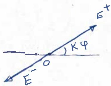
$$\begin{aligned} |E_T| &= E^+ - E^- = \frac{Kq}{R^2} \left( \frac{\sin(K+1)\phi - \sin K\phi}{\sin\phi} \right) \\ &= \frac{Kq}{R^2} \left( \frac{2\sin\frac{\phi}{2} \cos\frac{2K+1}{2}\phi}{2\sin\frac{\phi}{2} \cos\frac{\phi}{2}} \right) \\ &= \frac{Kq}{R^2} \left( \frac{\cos\frac{N+1}{2}\phi}{\cos\frac{\phi}{2}} \right) \quad \text{و } E_T \text{ ای } = K\phi = \frac{N}{2}\phi \end{aligned}$$
